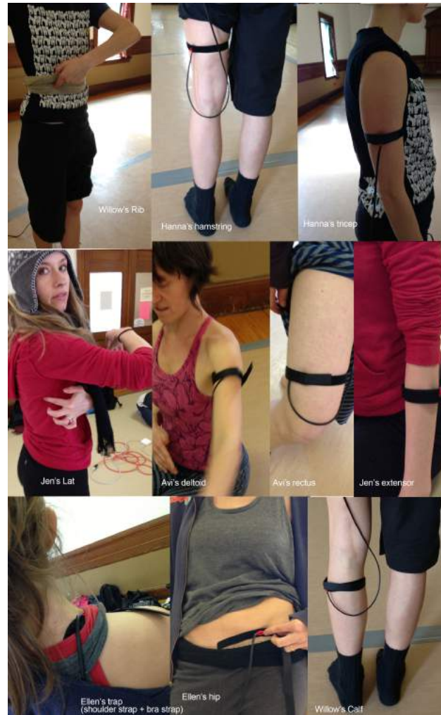
Fig. 30 – Sensor placement on each dancers body during testing phase (2013)
